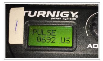
Use the "Adjust" knob on each servo tester to move its respective servo. Using both in unison will allow you to move the HP to specific positions. Feel free to mess around and get a feel for it.
